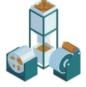
The mulcher is a machine that breaks the wood into tiny chips.
